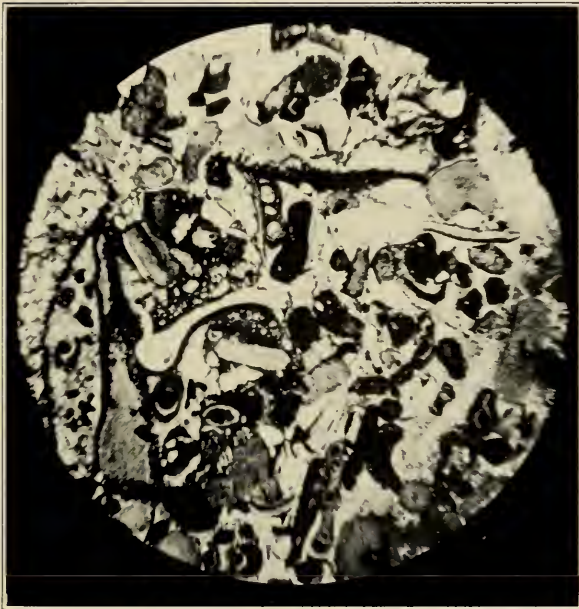
PLATE LXIII.—Photomicrograph.—Dull-red, Union Limestone. x 20. (Photo. by A. Berg and W. E. Rumsey).
